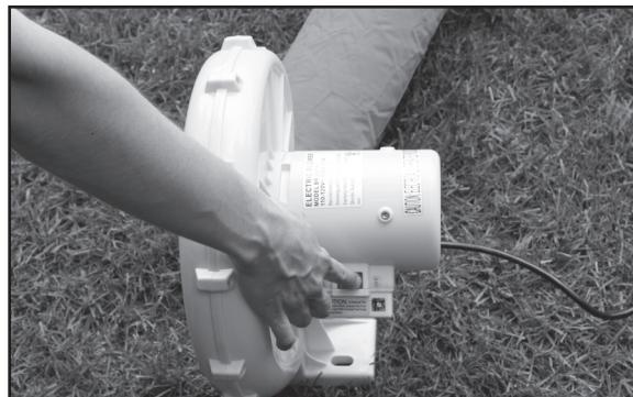
A GFCI device needs to be used (if your blower is not already equipped with one). Do not use an extension cord to power the blower. Keep the blower and power cord away from water. Plug in and start the blower; your unit will inflate within a couple minutes. You must leave the blower running the entire time the inflatable is being used. You will hear air "breathing" out of seams and fabric. This is intentional to allow air to escape.
